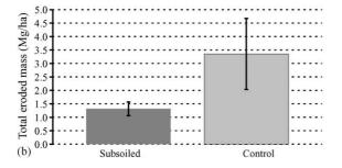
Fig. 4. Eroded material averages and standard errors (n=4) from simulated rainfall plots. (A) Mass of eroded soil (kg) mass from plots at 5 min intervals following initiation of flow. Letters above incremental data points indicate significance of difference between treatments: a,  $\alpha \leq 0.01$ ; b,  $\alpha \leq 0.05$ ; c,  $\alpha \leq 0.10$ . (B) Total eroded material (Mg/ha) from  $51 \pm 1$  mm of simulated rainfall.
