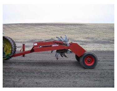
Fig. 2. Rotary subsoiler in transport position.
