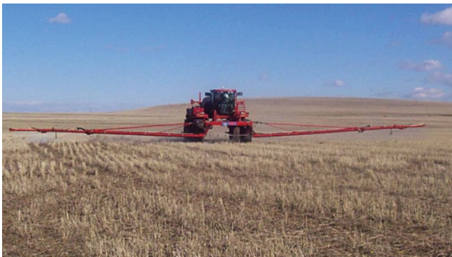
Figure 2. Weed control applications in commercial-sized fields are often made with large, self-propelled sprayers capable of treating 800 acres or more in a single day.
